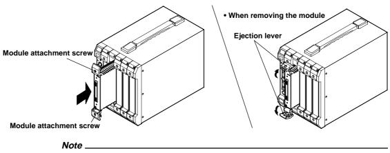
When synchronizing multiple isolated digitizer modules for measurement (module linking), install them in adjacent slots.
