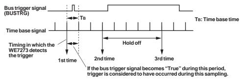
In addition, the WE7273 can output a bus trigger signal upon detecting a trigger within the module, and receive the results of the AND/OR computation on the bus to trigger the actual trigger operation.
