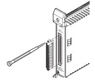
When connecting the input signal wire to the clamp type terminal, loosen the screw holding down the clamp, insert the input signal wire into the opening, and then tighten the screw.
